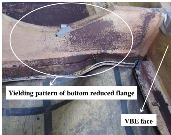
Figure 2 Yielding pattern at the end of intermediate HBE
